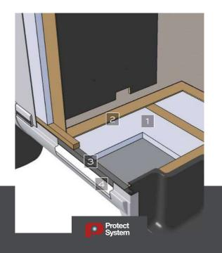
The insulating XPS Styrofoam (30 mm of Styrofoam either side and in the floor) is renowned for its great thermal and acoustic insulating properties, water-resistance and lightness.
